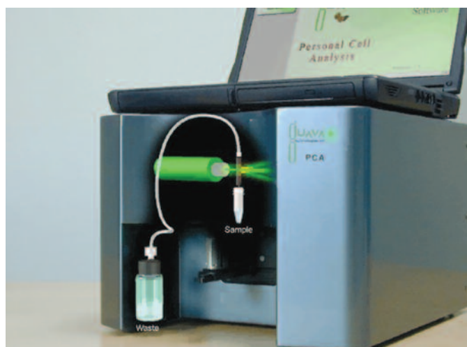
Inside the EasyCyte – sperm cells travel automatically through a microcapillary system to be analysed.
