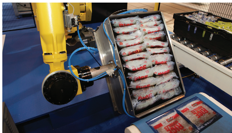
Pacepacker's Shingle Tray Loader addresses the challenges of vertically stacking flexible packs.
