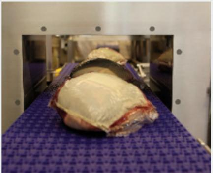
Being IP69K rated, the new range is resistant to water ingress, ensuring long-term reliability and performance heavy washdown meat processing environments.
