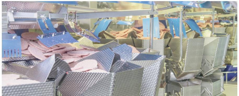
The accuracy of the new Ishida CCW-RS multihead weighers – 14-head, waterproof models, each equipped with five litre hoppers – means that McKey now achieves an approximate deviation from target weight of just 1g in each carton.
