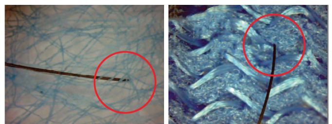
Fig. 2. 500 x magnification of human hair against a mob cap, left, and KleenCap, right.
