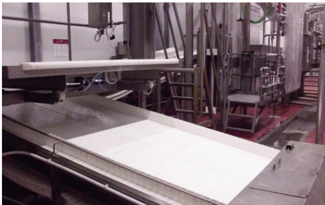
Pouchcasing package removal station.
