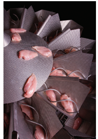
The incorporation of rotating screws into a multihead weigher provide the automated and controlled feed of product for accurate weighing.
