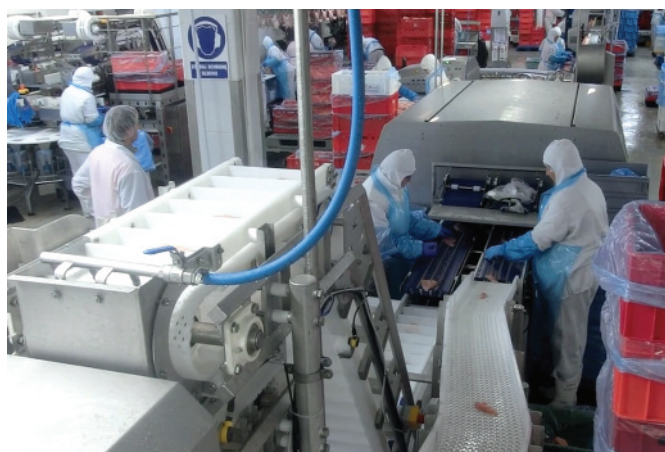
A grader groups the portioned meat into batches.
