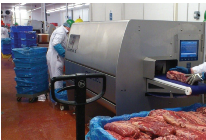
Loading high volumes of the primals into the portion cutter.
