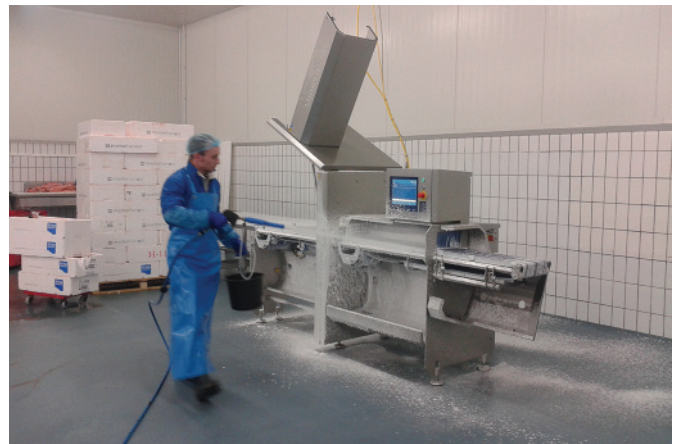
The open structure of the equipment allows complete sanitising of the portion cutter.
