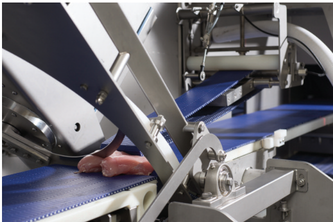
The cutting angle can be changed over 30° or 45° from its vertical position in a few seconds.
