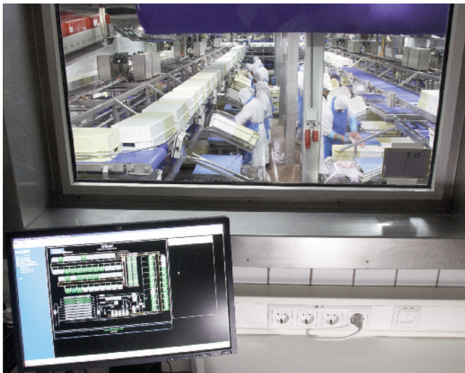
The SFK LEBLANC traceability software tracks and traces products throughout the entire production process.
