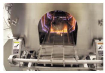
Using the flame tunnel processors. Simply take the cooked and chilled whole poultry or meat products from the chiller and place them on a belt that moves the products through an enclosed flame that will colour, sear and surface-pasteurise the products so that they are ready for immediate packaging.
