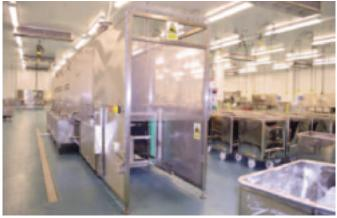
The ET 75 tunnel washer is designed to offer a continuous, in-line washing solution for buggies, trays, bins and other containers that not only cleans and sanitises thoroughly, but also offers a wide range of options, including various different heating methods, such as gas, steam coils, live steam injection and electric.
