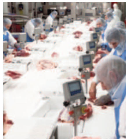
Yield, throughput, quality and other KPIs for each individual operator is registered and monitored online.
