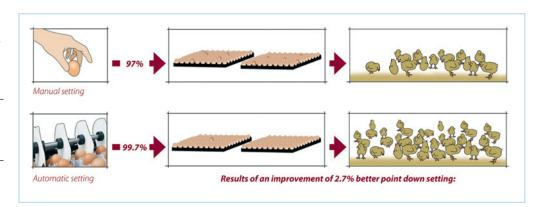
Point-down setting can be done manually, but ideally, this is an automated process. Automation in this case does not only mean saving labour. Actually, even more importantly moving to an automated point-down setting will reduce inconsistencies and prevent errors.
