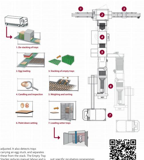
carrying an egg stuck, and separates Stacker reduces manual labour and is suitable for paper and plastic trays.
