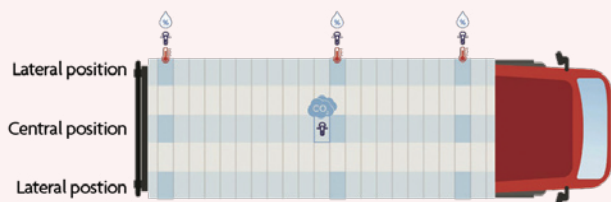
Fig. 1. Aerial view of the truck, highlighting the centre and lateral rows. The coloured squares represent the boxes with temperature and RH probes. The position of the CO 2 probe is also shown.
