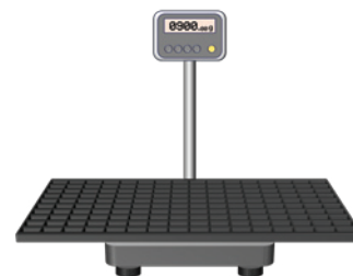
Fig. 3. Weigh the tray with eggs at transfer and then weigh the tray without the eggs.
