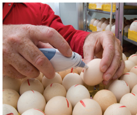
Fig. 3. Monitoring eggshell temperature using (a) an infrared ear thermometer, (b) a thermal imaging camera and (c) dataloggers.
