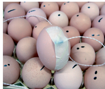
Fig. 3. Monitoring eggshell temperature using (a) an infrared ear thermometer, (b) a thermal imaging camera and (c) dataloggers.
