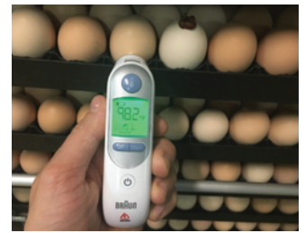
The difference in heat emission between exothermic live embryos and rotten eggs.
