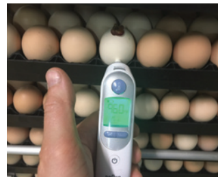
The difference in heat emission between exothermic live embryos and rotten eggs.
