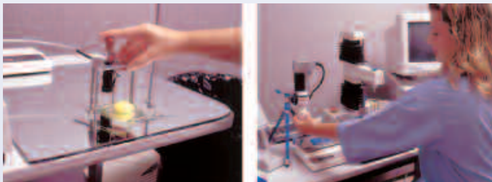
Left, the height of the thick white is measured and recorded automatically as a probe is lowered into the albumen. Right, shell colour is measured for both white and brown shelled eggs.
