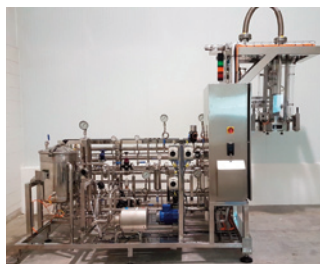
The new HRS Asepticblock Mini provides a compact and complete solution for producing small volumes of aseptic products.
