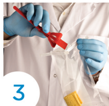
STEP 3 Press on the bottom of the hands to gently release the sponge into the sterile sampling bag.
