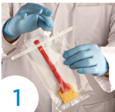
STEP 1 Remove the tear-off strip and carefully take the Sani-stick by the handle.
