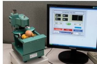
Fig. 1. Components of the new shell quality evaluation, from left to right: breaking strength at the equator (BS e ) and between the poles (BS p ), and the Acoustic Egg Test (AET).
