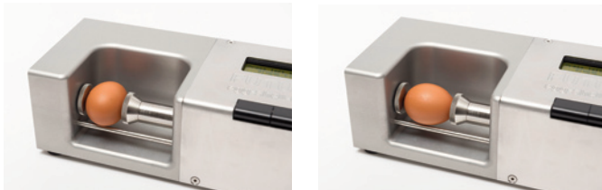
Fig. 1. Components of the new shell quality evaluation, from left to right: breaking strength at the equator (BS e ) and between the poles (BS p ), and the Acoustic Egg Test (AET).
